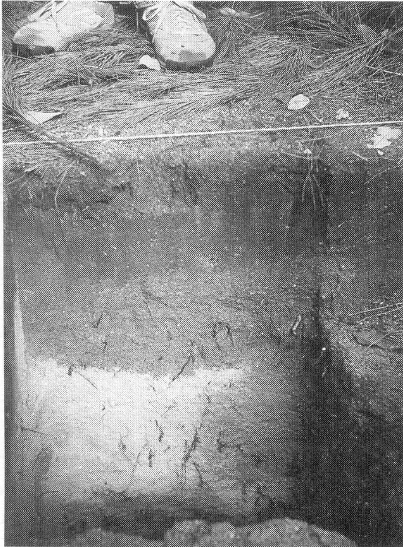
Wetting front in a sandy soil exposed after intense rain (from Dingman, 1994).
